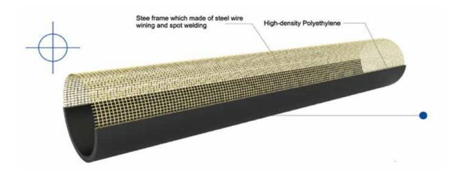
Inner and outer polyethylene layers: special pipe-grade high-density polyethylene is used as the main material. All polyethylene has passed the strict inspection of GB/T 18252, and the hygienic performance meets the requirements of international standards such as GB/T17219. The polyethylene layer has the characteristics of hygiene, strong conveying capacity, excellent resistance to slow crack growth, excellent impact resistance and high temperature resistance.
