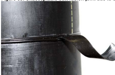
Figure 39: Unacceptable butt fusion joint due to contamination captured in the joint
