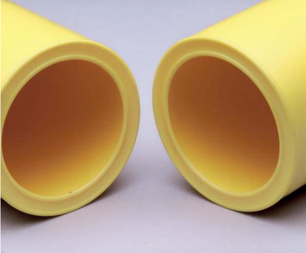
Figure 41: Unacceptable cupped surfaces after heat soak cycle
