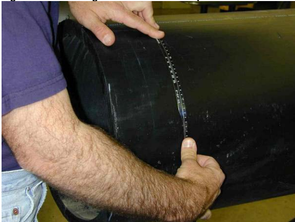
Figure 47: Measuring Diameter with a Pi Tape
