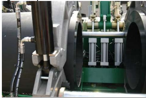
Figure 32: Pipe Cleaned and Secured for Butt Fusion
