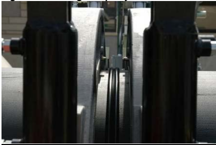
Figure 36: Joining of Pipe by Butt Fusion
