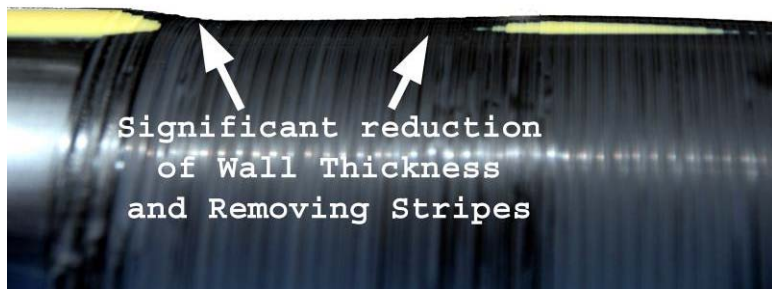
Figure 69: Over Scrape Unacceptable – Possible Causes: Incorrect Scraper, Poorly Maintained Scraper, Excessive Number of Passes with Scraper and Ineffective Evaluation of Scraping
