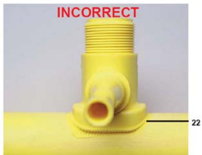
22. Insufficient melt and misaligned
