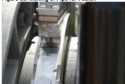
Figure 35: Melting of Pipe for Fusion
