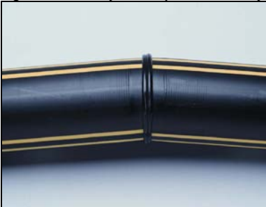
Figure 42: Visually unacceptable mitered joint
