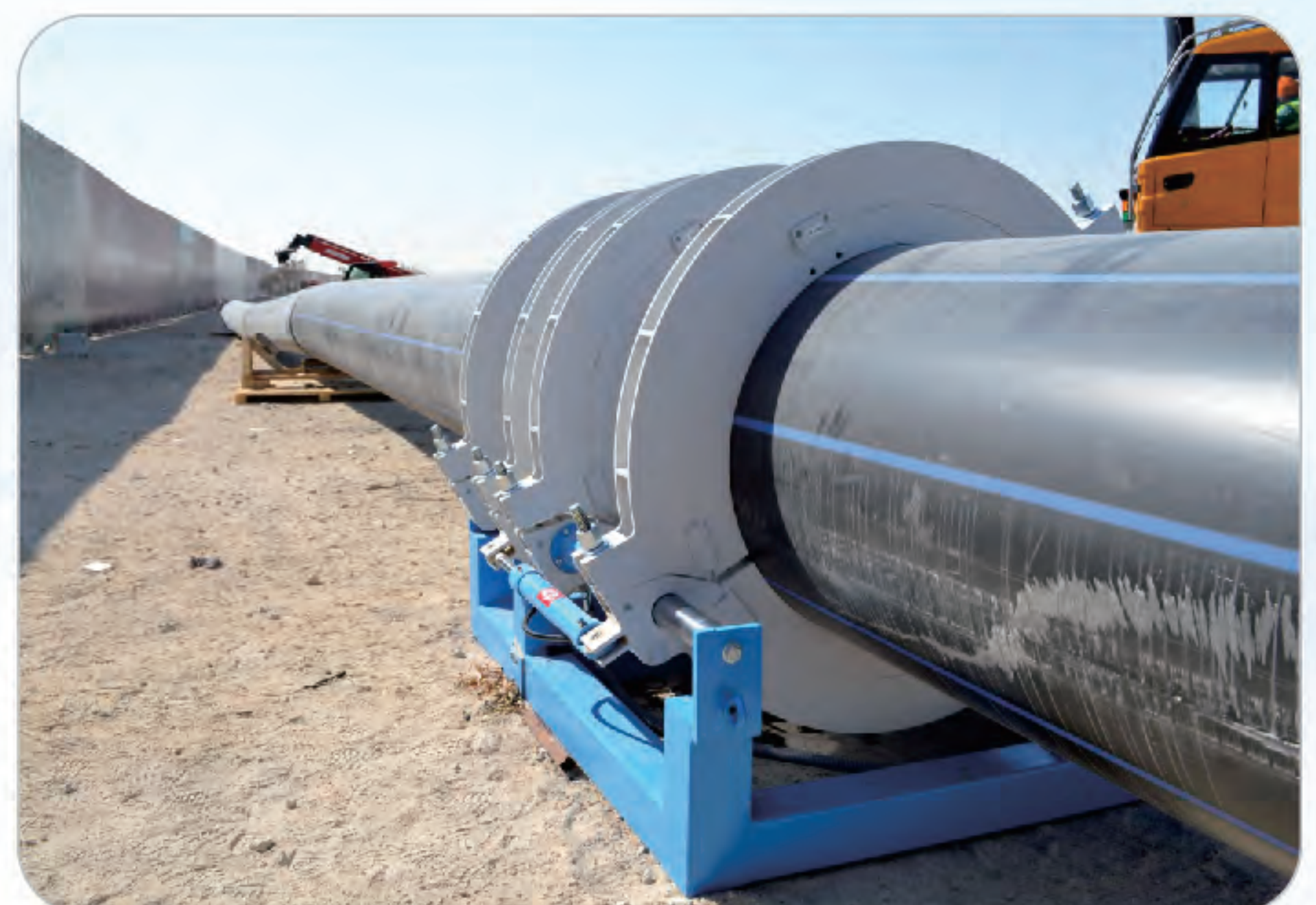
Petroleum Engineering: Corrosion-resistant piping system for UAE petrochemical plant DN1000, HDPE Pipe
